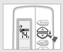
3 To adjust the temperature, press the buttons one or more times until the required temperature is displayed. Possible temperatures are between 65°F(18°C) and 86°F(30°C) inclusive.
